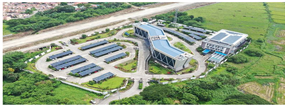
Aerial view of the MPT South Hub, featuring 1,184 solar panels that generate about 97% of the building's energy needs. The facility also has a rainwater harvesting system that reduces water use by 10%, along with EV charging stations for company electric vehicles.
